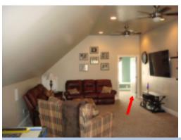
The door to the 3rd floor bedroom drags and is difficult to open or close. This condition could indicate improper installation. The door needs repair to ensure that the door closes securely and operates properly. A general repair specialist or licensed general contractor should be consulted for evaluation and repair.
